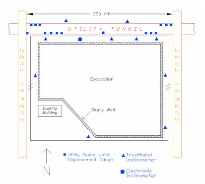
FIG. 4. Instrumentation plan for excavation near utility tunnel
